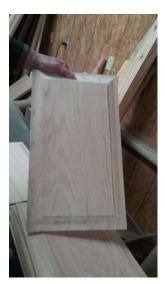
Like many <u>Craftsman</u> designs this bed features raised panel construction... but here there's a twist. Here the headboard includes raised panels set in a dado that serve as a design element. See the pic at above-left.
