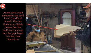
The process of mounting the rough-cut shelves to the spoil board and then cutting to the final dimension is know in the trade as "pattern sawing" and has been around for an exceptionally long time. Following this process, you will repeatedly get shelves that are the same repeatedly. One other
