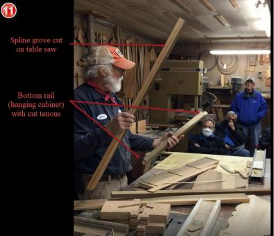
The angle you want on these boards is 22 ½ degrees. This joint is not going to stay lined up down the length of the board without a spline. John uses 1/8" Baltic Birch for the spline. He usually gets it from York Lumber Company and comes in a 5' x 5' sheet. You can make the kerf with your saw blade on the table saw. Remember you are also going to have a top piece, a middle piece and a bottom. The best joinery for this is mortise and tenon and you want to cut these prior to case assembly and glue
