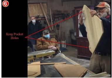
If you do not have a Kreg Jig, you can use the marks made by the screws to hold the stock as guides for drilling the pilot holes.
