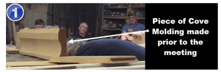
Cove Molding is usually the result of grouping and joining several different molding pieces into one final product. The part of the group picture #1 represents is shown in Picture #2.
