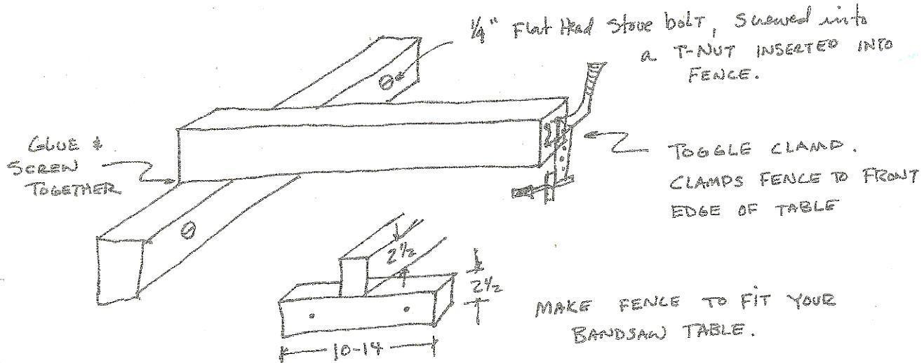
NOTE: VERY FEW BANDSAWS ACTUALLY CUT PARALLEL WITH THE TABLE. A FENCE MUST BE ADJUSTABLE TO THE BANDSAW'S "ANGLE OF DRIFT". THE STOVE BOLTS IN THE T-NUTS ALLOW YOU TO ADJUST THE FENCE TO THE "A.O.D." TO FIND YOUR SAW'S A.O.D., DRAW A STRAIGHT LINE ACROSS THE CENTER OF A BOARD APP. 10X10. MAKE A FREE HAND CUT ON THIS LINE, STOPPING MIDWAY. WITHOUT MOVING THE BOARD, MARK THE ANGLE ALONG ONE EDGE W/ A PENCIL. SET YOUR FENCE TO THIS ANGLE. IT WILL PROBABLY NEVER CHANGE.
